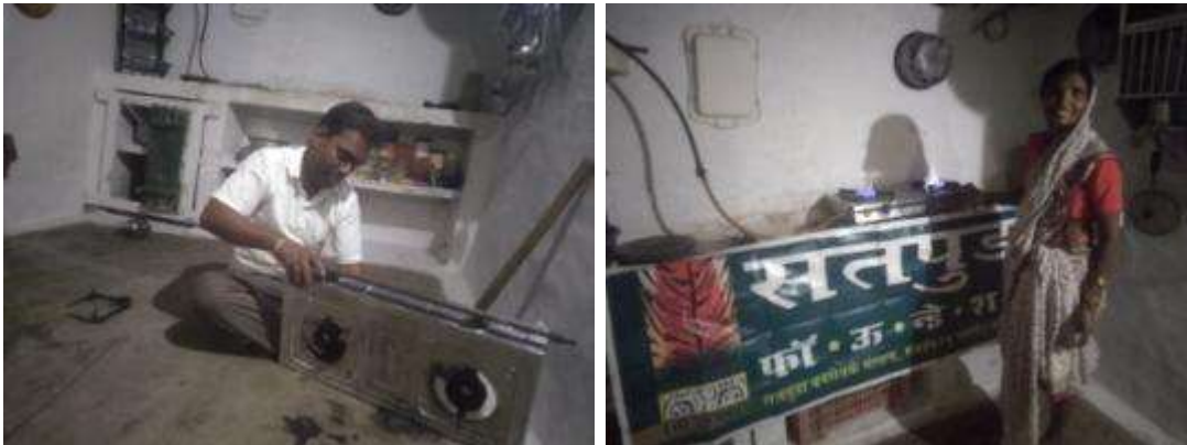
Turiya – Niranjana undertaking repair of a faulty biogas stove (left); stove after being repaired (right)
