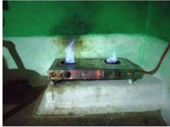
Bio-gas stove being repaired by Niranjan (left) and the unit working after repair (right)
