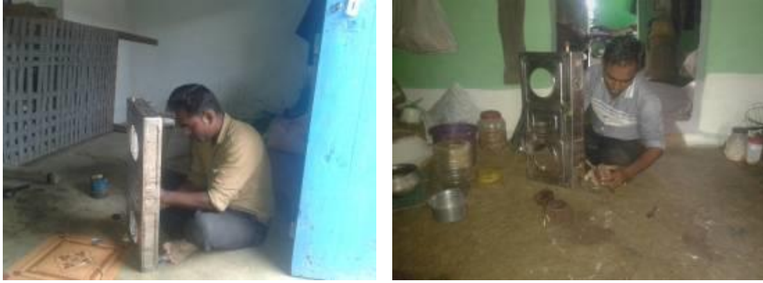
Nirranjan repairing biogas stove units in Aamajhiri village
